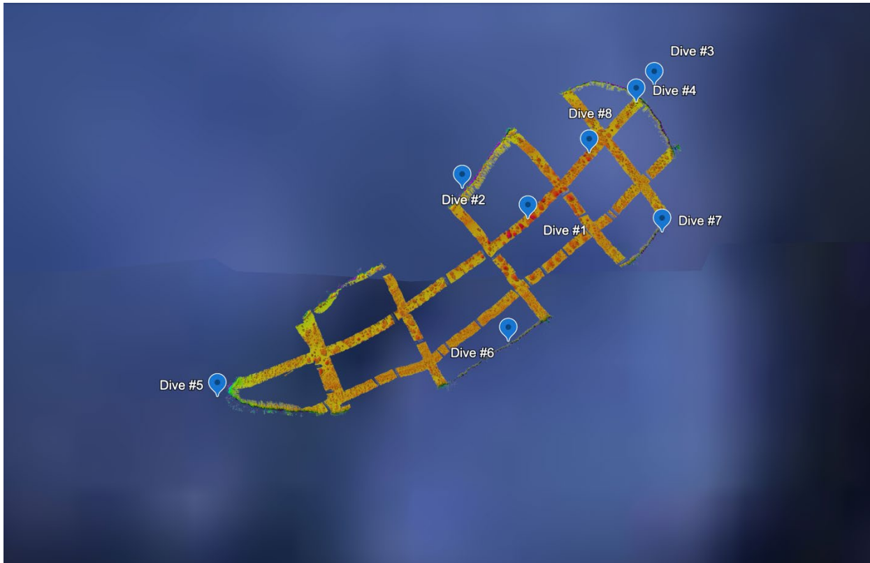
Fig. 2. Bathymetric map created using side-scan sonar technology of Pickle Bank, created by Prof. Arthur Trembanis (U. Delaware). Marker indicate the locations of each dive where surveys were conducted.
